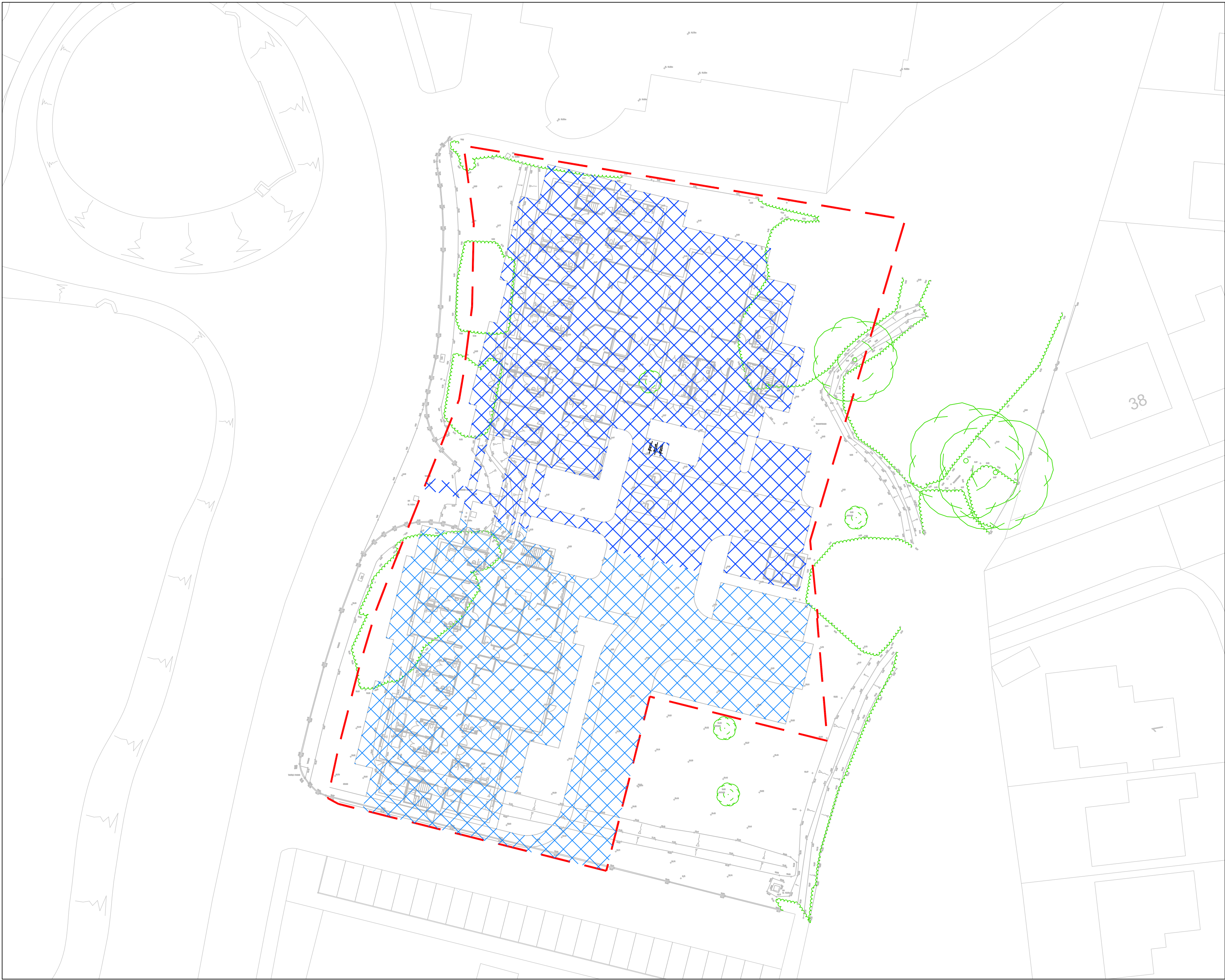
PROPOSED / EXISTING IMPERMEABLE AREA APPROX SCALE 1:333
